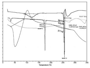
Figure 7: DSC thermograms of A) Acyclovir B) cholesterol C) PC D) optimized proliposome gel formulation (ACVPL2).
