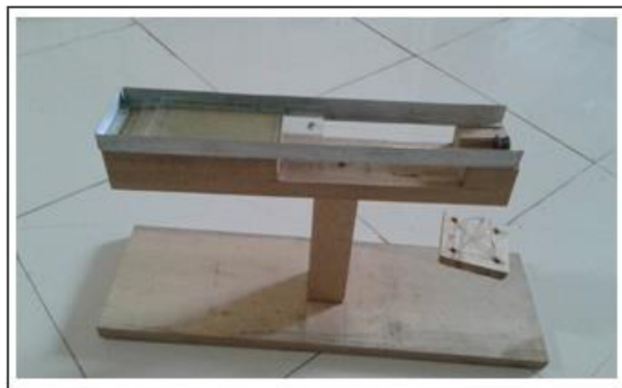
Figure 1: Fabricated apparatus for spreadability.
