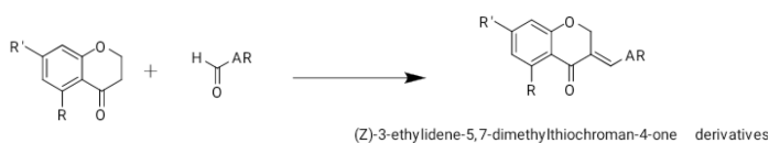
Scheme 1: Reagents and conditions (i) Pyrrolidine, dry MeOH, rt, 1-24h or 120C, 1h
