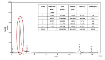
Figure 1: HPLC Chromatogram of Methanol fraction showing various peaks and other characteristics of purified fraction (Detector A Ch1 254 nm).
