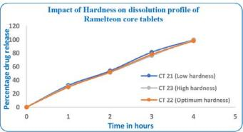
**Figure 4:** Impact of Hardness on dissolution profile of Ramelteon core tablets. The y-axis represents % drug release and the x-axis denotes times in hours. Data represent mean  $\pm$  standard deviation, n = 3.
