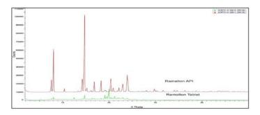
**Figure 7:** Overlay XRD diffractogram of the Ramelteon API and the finished dosage form.
