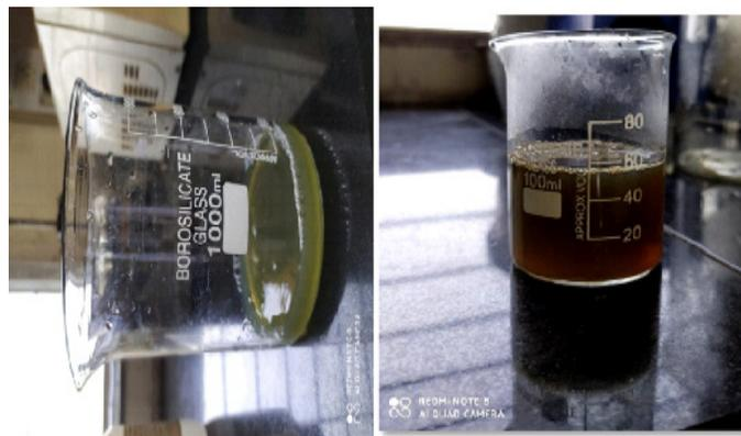
**Figure 1:** a) Mixture of AgNO<sub>3</sub> solution and leaf extract. b) Synthesis of AgNP's and colour change of mixture after microwave irradiation.
