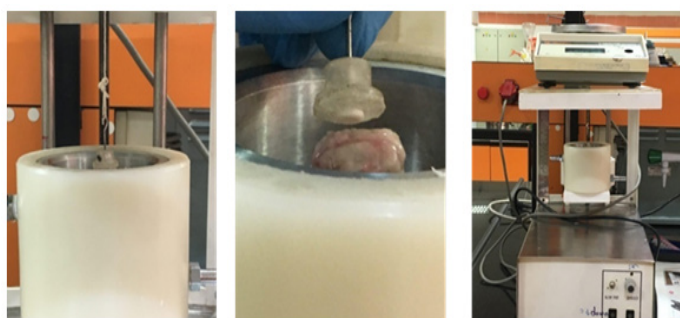
Figure 2: Mucoadhesive strength testing apparatus.
